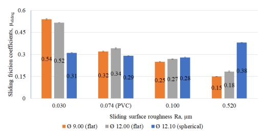
Fig. 3. Sliding friction coefficient  $\mu_{slide}$  values for each sliding body type on sliding planes with different surface roughness
