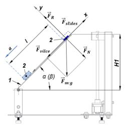
Fig. 1. Force vector scheme: 1 - sliding plane; 2 - slide body;  $\alpha$  - static friction angle;  $\beta$  - sliding friction angle;  $\vec{F}_N$  - normal force (downforce);  $\vec{F}_R$  - support reaction force;  $\vec{F}_{vilce}$  - traction force;  $\vec{F}_{slīdes}$  - sliding friction force;  $\vec{F}_{mg}$  - gravity force;  $H_I$  - elevated height of sliding plane
