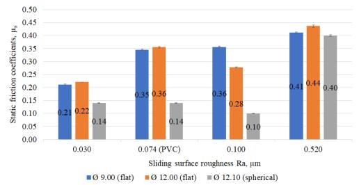
Fig. 5. Dependence of static friction coefficient  $\mu_s$  on sliding plane roughness *Ra* for each type of sliding bodies
