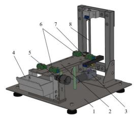
Fig. 2. Tribometer equipment overview: 1 - base with adjustable supports; 2 - sliding plane;
